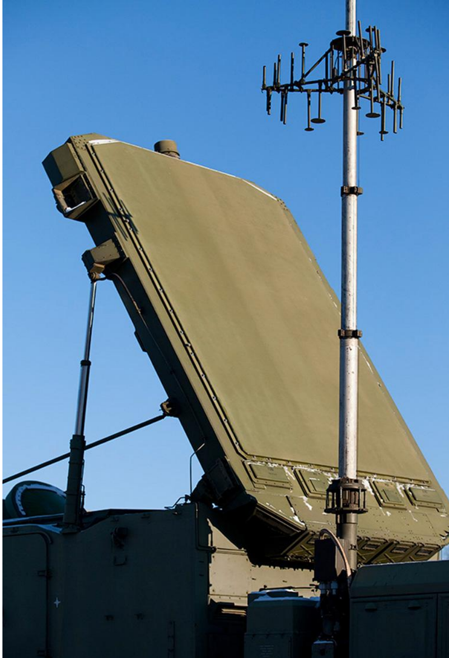
92N6E Grave Stone with space feed primary antenna deployed, and telescoping datalink mast elevated. Note the auxiliary apertures used for sidelobe cancelling and interferometry along the base of the main transmissive array.
