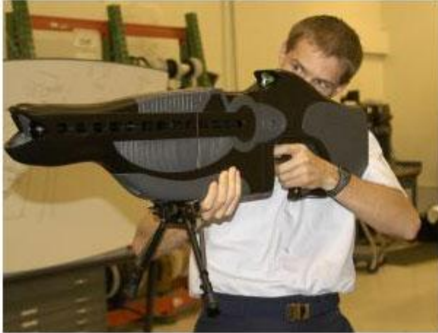
A modified version of this laser rifle created to dazzle enemies by the US Air Force has been adapted by the Department of Justice to inflict pain from a distance (Image: US Air Force)
