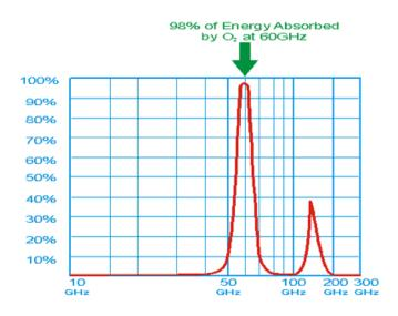
Figure 1 illustrates the atmospheric absorption for millimeter wave frequencies. At the millimeter wave frequency of 60 GHz, the absorption is very high, with 98 percent of the transmitted energy absorbed by atmospheric oxygen. While oxygen absorption at 60GHz severely limits range, it also eliminates interference between same frequency terminals.
