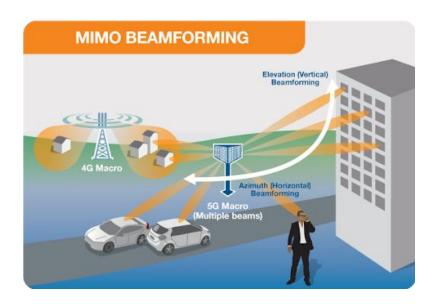
5G also employs new technologies (e.g., active antennas capable of beamforming; phased arrays; massive multiple inputs and outputs, known as massive MIMO) which pose unique challenges for measuring exposures.
