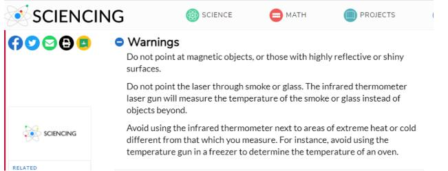
Warnings: Do not point at magnetic objects, or those with highly reflective or shiny surfaces. Do not point the laser through smoke or glass. The infrared thermometer laser gun will measure the temperature of the smoke or glass instead of objects beyond. Avoid using the infrared thermometer next to areas of extreme heat or cold different from that which you measure. For instance, avoid using the temperature gun in a freezer to determine the temperature of an oven.
